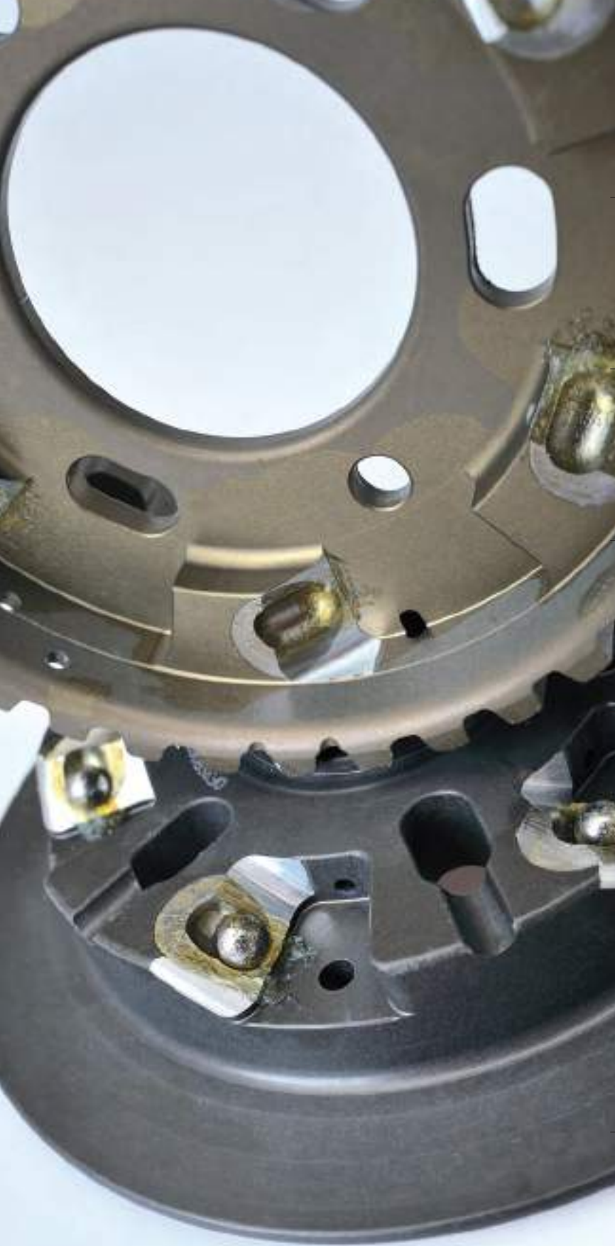
rasamenti molla primaria e secondaria primary and secondary support
